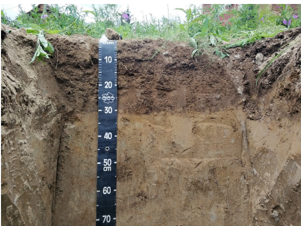
Figure 3. Profile of Plaggic Podzol (Turbic)
